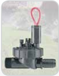
Male x Barb Specifically designed for use with polyethylene piping systems. Requires fewer fittings and allows faster installation. Choice of ¾", 1", or 1¼" barb outlets for compatibility with different systems.
