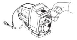
Always ensure your pump casing is full of water prior to initial start up or the pump seal may be damaged.
