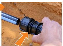
Ensure 2 threads are showing and simply slide the pipe in until the first point of resistance is felt.
