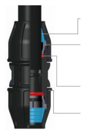
Split ring bites into pipe. High internal pressure or tensile load causes the split ring to bite further into the pipe.
