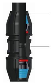
Clearance between pipe and fitting allows for easy insertion of the pipe.
